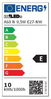
Depth of the light source [mm]: 60 Colour rendering index: 80 Chromaticity coordinates (x): 0.38 Chromaticity coordinates (y): 0.38 Claim of equivalent power [W]: 75 R9 colour rendering index value: 10 Survival factor:  $\geq 0.9$ The lumen maintenance factor: 0.93
