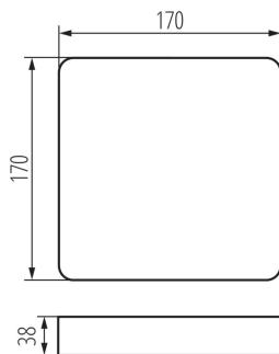
Kanlux TAVO FRAME allows surface mounting of Kanlux TAVO LED panels in 12W and 18W versions. The tightness of the panels after mounting is IP20.
