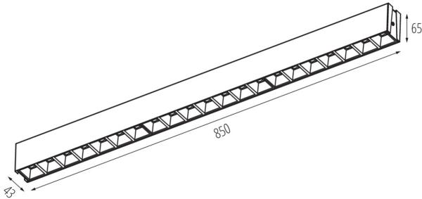
**PARAMETERS FOR LED AND OLED LIGHT SOURCES:****Correlated colour temperature [K]: 3000****Colour consistency in McAdam ellipses : ≤6****Colour rendering index: 80****LOGISTIC DATA:****Unit of measurement: unit****Packaging method: 1****Number of units in the secondary packaging : 1****Number of units in the packaging : 1****Net unit weight [g]: 1470****Grammage [g]: 1870****Weight of a cardboard box [kg]: 1.87**
