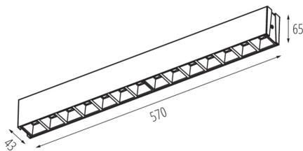
**PARAMETERS FOR LED AND OLED LIGHT SOURCES:****Correlated colour temperature [K]:** 3500**Colour consistency in McAdam ellipses :** ≤6**Colour rendering index:** 80**LOGISTIC DATA:****Unit of measurement:** unit**Packaging method:** 1**Number of units in the secondary packaging :** 1**Number of units in the packaging :** 1**Net unit weight [g]:** 1080**Grammage [g]:** 1300**Weight of a cardboard box [kg]:** 1.3
