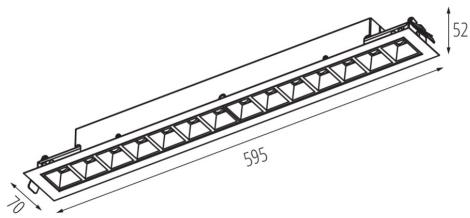
**PARAMETERS FOR LED AND OLED LIGHT SOURCES:****Correlated colour temperature [K]:** 3000**Colour consistency in McAdam ellipses :** ≤6**Colour rendering index:** 80**LOGISTIC DATA:****Unit of measurement:** unit**Packaging method:** 1**Number of units in the secondary packaging :** 1**Number of units in the packaging :** 1**Net unit weight [g]:** 1000**Grammage [g]:** 1180**Weight of a cardboard box [kg]:** 1.18
