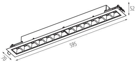
**PARAMETERS FOR LED AND OLED LIGHT SOURCES:****Correlated colour temperature [K]:** 3500**Colour consistency in McAdam ellipses :** ≤6**Colour rendering index:** 80**LOGISTIC DATA:****Unit of measurement:** unit**Packaging method:** 1**Number of units in the secondary packaging :** 1**Number of units in the packaging :** 1**Net unit weight [g]:** 1000**Grammage [g]:** 1180**Weight of a cardboard box [kg]:** 1.18
