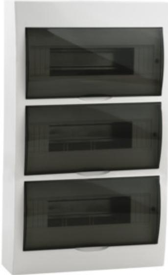
DB series switchboards, meeting the requirement for heat resistance at the temperature of 650°C, can be used on non-flammable surfaces only (e.g. full solid walls made of non-combustible materials). They cannot be used on flammable surfaces (e.g. plasterboard, wood boards, etc.), on the so-called "hollow walls" or on technical sections.
