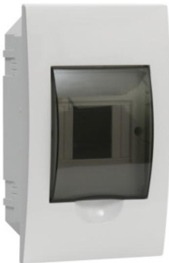
DB series switchboards, meeting the requirement for heat resistance at the temperature of 650°C, can be used on non-flammable surfaces only (e.g. full solid walls made of non-combustible materials). They cannot be used on flammable surfaces (e.g. plasterboard, wood boards, etc.), on the so-called "hollow walls" or on technical sections.
