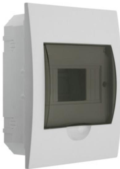
DB series switchboards, meeting the requirement for heat resistance at the temperature of 650°C, can be used on non-flammable surfaces only (e.g. full solid walls made of non-combustible materials). They cannot be used on flammable surfaces (e.g. plasterboard, wood boards, etc.), on the so-called "hollow walls" or on technical sections.
