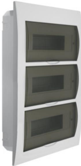
DB series switchboards, meeting the requirement for heat resistance at the temperature of 650°C, can be used on non-flammable surfaces only (e.g. full solid walls made of non-combustible materials). They cannot be used on flammable surfaces (e.g. plasterboard, wood boards, etc.), on the so-called "hollow walls" or on technical sections.
