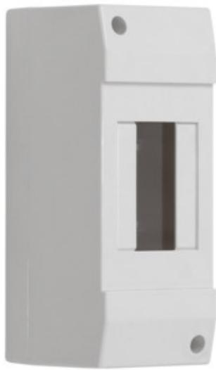
DB series switchboards, meeting the requirement for heat resistance at the temperature of 650°C, can be used on non-flammable surfaces only (e.g. full solid walls made of non-combustible materials). They cannot be used on flammable surfaces (e.g. plasterboard, wood boards, etc.), on the so-called "hollow walls" or on technical sections.
