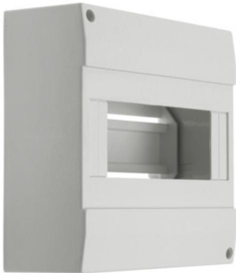
DB series switchboards, meeting the requirement for heat resistance at the temperature of 650°C, can be used on non-flammable surfaces only (e.g. full solid walls made of non-combustible materials). They cannot be used on flammable surfaces (e.g. plasterboard, wood boards, etc.), on the so-called "hollow walls" or on technical sections.
