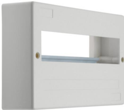
DB series switchboards, meeting the requirement for heat resistance at the temperature of 650°C, can be used on non-flammable surfaces only (e.g. full solid walls made of non-combustible materials). They cannot be used on flammable surfaces (e.g. plasterboard, wood boards, etc.), on the so-called "hollow walls" or on technical sections.
