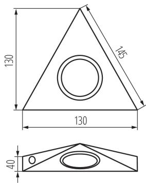
The Kanlux ZEPO series of eyes is the lighting intended under cabinets, for example, above a table top in a kitchen. ZEPOs are available in a version with an OFF switch and without it. The holders require a power supply unit e.g. from the SET series. JC with G4 thread is a light source intended for the eyes.
