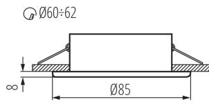
Kanlux MARIN means small and tight ceiling holders to be used in places with increased humidity. They can easily be placed in a bathroom above a mirror, in a kitchen or in a laundry.
