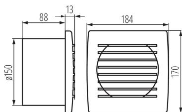
Kanlux CYKLON EOL series of fans is available in three sizes with diameter of 100, 120 and 150mm. They are made of plastic, in white colour. Their power is 19, 20 and 22W respectively. The number of rotations from each size comes to 2550/min.
