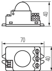
Kanlux ROLF JQ is a motion detector. The horizontal angle of the detector work comes to 360 degrees. You can set adjustments of the lighting time and light intensity level at which the detector works.
