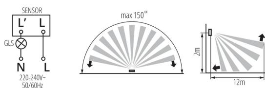
Kanlux MARID JQ is a motion detector whose maximum detection range comes to 12 metres. You can set adjustments of the lighting time and light intensity level at which the detector works. The detector can be activated by means of sound signal too.
