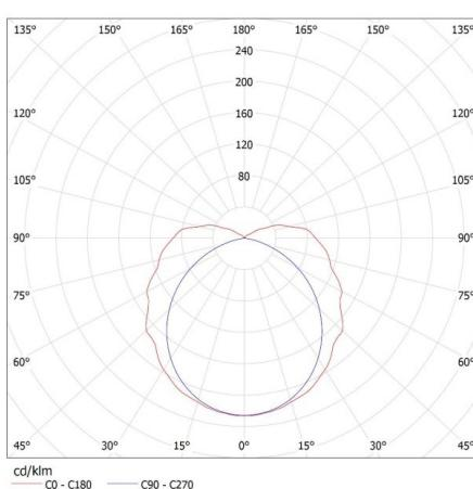
KANLUX S.A. (kat 22803) MAH PLUS-158/4LED/PC + GLASSv3 / LDC (Polar)
